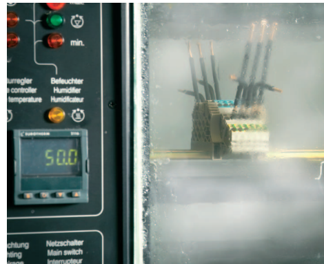
This test, in accordance with IEC 512-6-6 serves to assess the ability to withstand the effects of salt spray.
