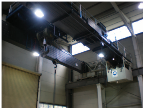
Aratiatia power station 100 tonne gantry crane
