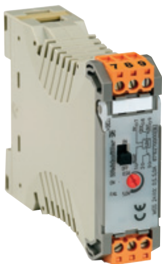
Weidmuller’s Waveguard senses a sudden rise in current, trips before fold-back or current limit occurs and isolates the faulty circuit
