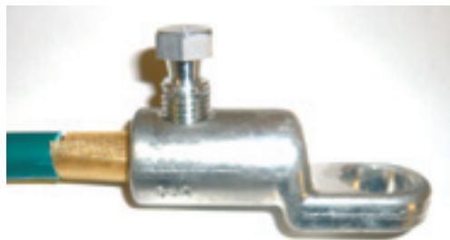
Brass gauze ensures the integrity of conductors by protecting the fine copper strands used in flexible and multi stranded cables
